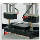
Fully automated impedance test of batteries in a production line. With **CMWTEC** DataManager, and a look-up process for the second Impedance test machine in order to verify the results of the first test.
