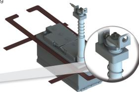
Behind the HRD follows the High Voltage Leakage Test section with self-adjustable test bars for checking the lid sealing and battery bottom box. These two test machines are used for final quality performance test and leakage test of the batteries. These units guarantee a high quality check of the battery at the end of the line. Connected to high-end digital electronic test devises, these units fulfill the OE requirements standards.
